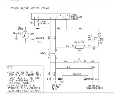
Note: Units are fitted with an extra terminal (P3) at the terminal block to provide a wiring connection point when used with JABC-1 Fresh Air Unit.
