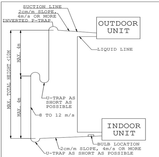
Figure 11: Piping Layout for Outdoor Below Indoor
