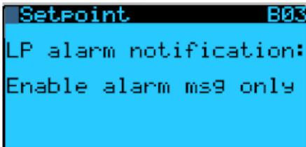
3. Press ENTER button to move cursor from 'home' position to the selection. Select the desired low pressure alarm notification setting by UP/DOWN arrows. Three types of LP alarm notification setting are available:
