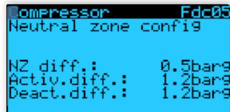
The rate at which the capacity decreases or increases depends on the times defaulted in masks Fdc07, Fdc08 and Fdc09. This means that the further away the suction pressure moves away from the Neutral Zone (either above or below), the quicker the controller will adjust the compressor capacity (**Figure 15**).
