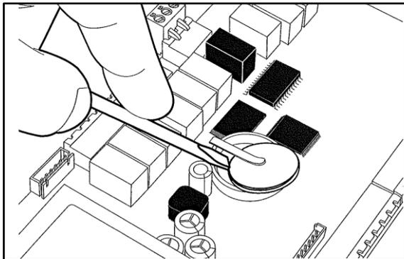
**The battery in the controller should be changed every three years.**
