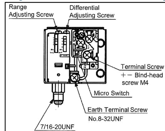
The pressure switch fitted to condensing units with auto reset for low pressure is factory preset to 1.0 bar cut-out. **Do not set low pressure cut-out lower than factory default setting.**
