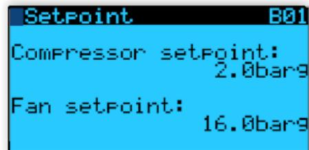
2. Using ENTER button, move the cursor from the 'home' position to the Compressor Setpoint and adjust value as required by using UP or DOWN buttons.
