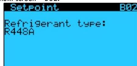
6. At screen B02, the Refrigerant Type can be selected. The default refrigerant is set as R448A.
