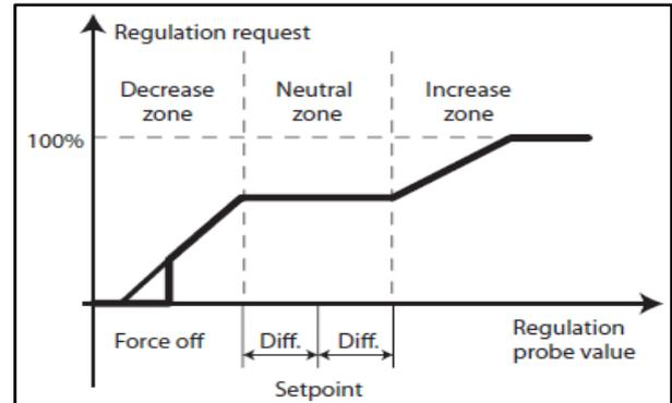
When the suction pressure falls inside the neutral zone (setpoint +/- differential), the capacity is stable and there is no loading or unloading of the digital scroll compressor.
