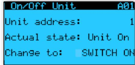
3. Press ENTER button to move cursor from home position to SWITCH OFF value. Switch Unit ON by using UP/DOWN arrows. Press ENTER button to confirm.
