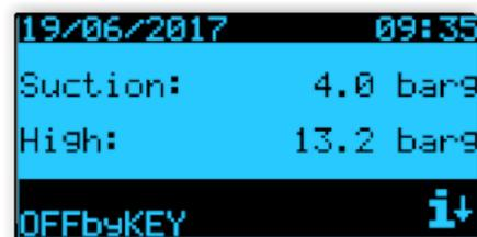
2. The low and high-sides conditions of the unit are displayed on screen M01. If **OFF by Key** is indicated in the lower box, it shows that the unit is switched OFF by the controller.
