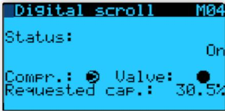
4. The symbols against Compressor and Valve change depending on their status (whether compressor is running or not and whether the capacity valve is open or closed). The percentage value will also change depending on the amount of capacity being provided at the current time.
