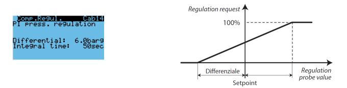
With proportional + integral control, the integral time is summed to the effect of proportional control, giving a null control error in steady operation. This type of control is illustrated in the following figure:
