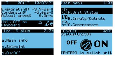
1. With controller Home screen displayed, Press PRG button to go Main Menu screen and select "A. Unit Status".
