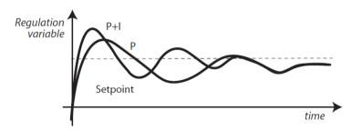
The integral action depends on time and the deviation from the set point. The integral time represents how fast integral control is implemented:
