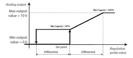
Fan control can be switched to be controlled by external temperature probe if fault discharge pressure transducer. Associated parameter to be changed on masks: Dg14, Dg15.
