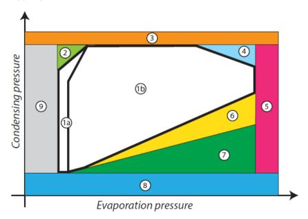
• Speed reduction when operation is beyond the high condensing pressure or high compression ratio limits, so as to return within the permitted operating zone.
